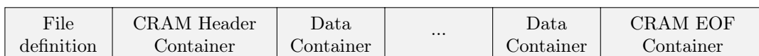
Figure 1: A CRAM file consists of a file definition, followed by a header container, then other containers.
